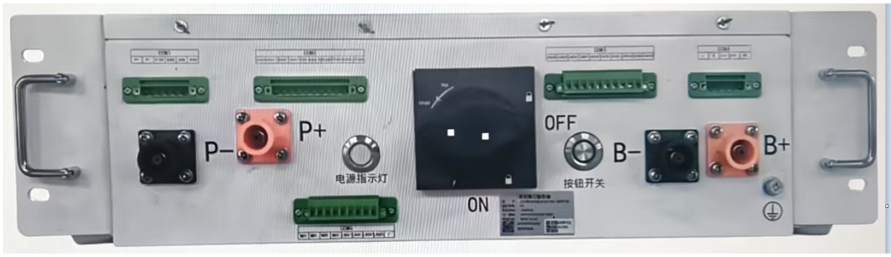
High Voltage Box (HVB)
